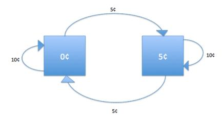
Note: We do not see the actions the vending machine takes represented on the state diagram. We only see the internal states and the observations that trigger new states.
